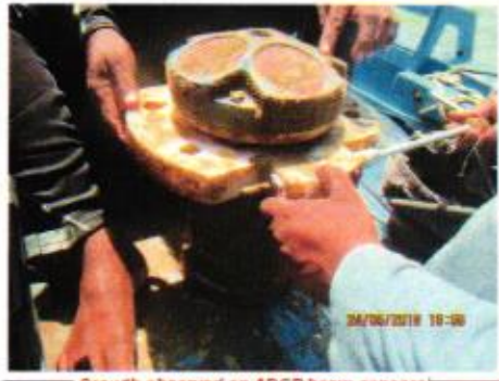
Growth observed on ADCP beam sensors
