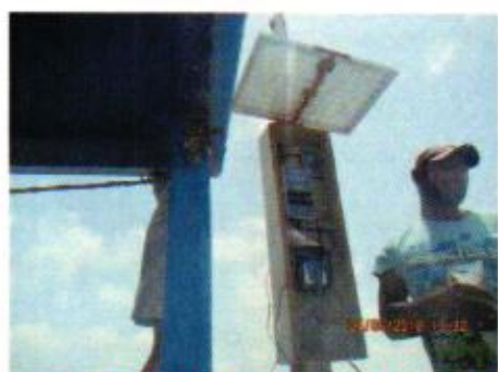
Sutronics USA GSPRS Modem for Telemetric Data Transfer
