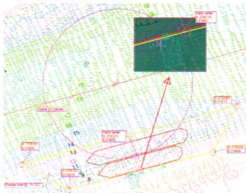
Figure 4.3: Jetty Location Respect to the Middle of the Channel (Ref.[12])
